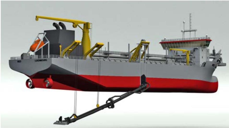
**Figure C.2.3.2 Typical trailer suction hopper dredge** (sediment is drawn in by the draghead and placed into the hopper in the vessel hull. The vessel is self-propelled and discharges the dredged material at the DMPA through bottom discharge gates)
