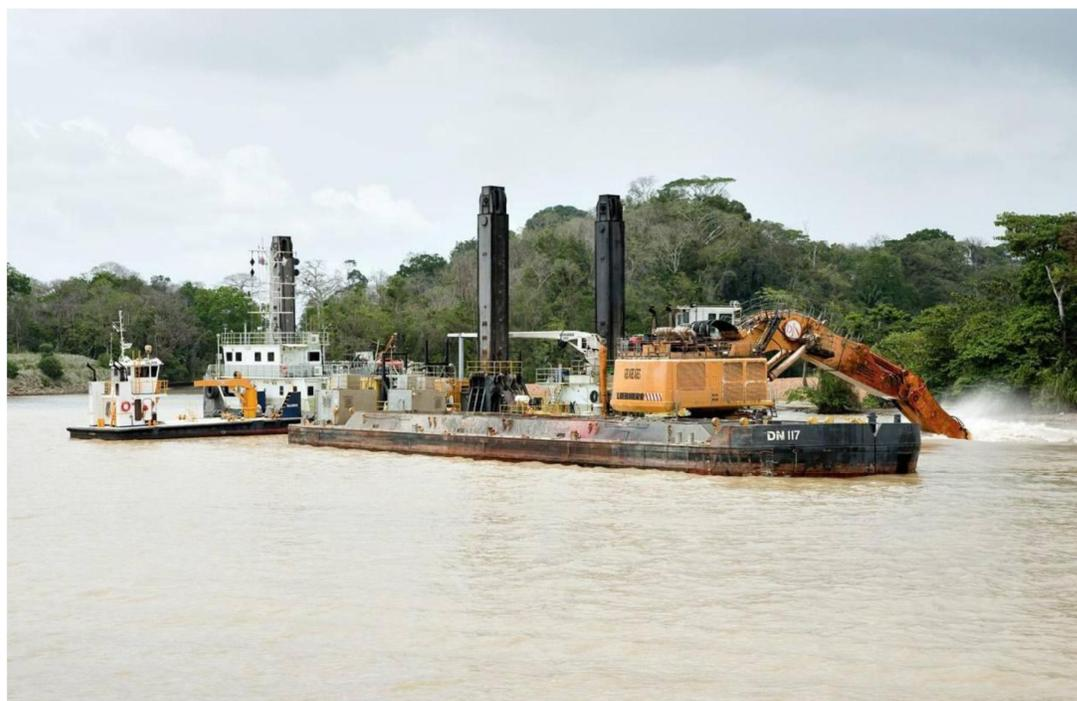
**Figure C.2.3.4 Typical backhoe dredge** (mechanically excavates material using a bucket at the end of the excavator arm and places it in a self-propelled hopper barges which are moored alongside for transport of the dredged material to the DMPA. The dredger is anchored using spud piles and manoeuvred by a tug).
